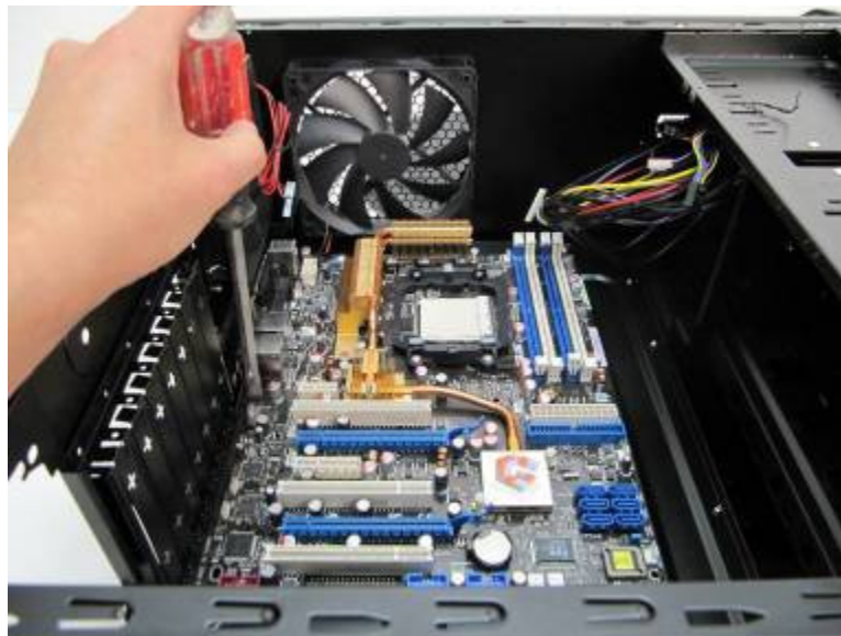
Step 5: Screwing in the motherboard after standoffs are installed
